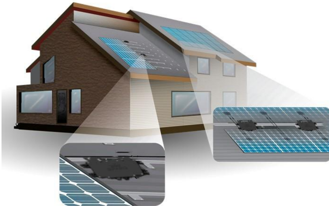
Figure 1: Typical roof-top micro inverter home installation.
